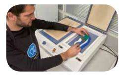
Thermoforming the selected OPCT<sup>®</sup> on the positive cast\*
