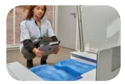
Use the Structure Sensor and an iPad to scan the vacuum bag imprints
