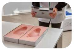
or use the Structure Sensor and an iPad to scan the imprint box prints
